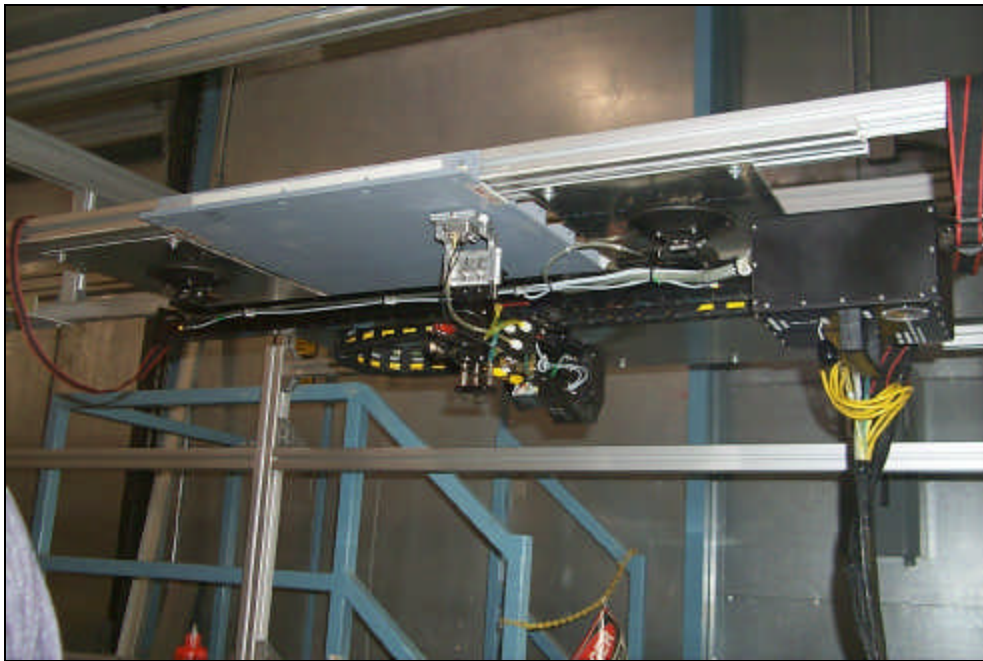
Figure 3.1. View of the dual transducer probe and automated scanner system on a sample panel during the validation experiment.
